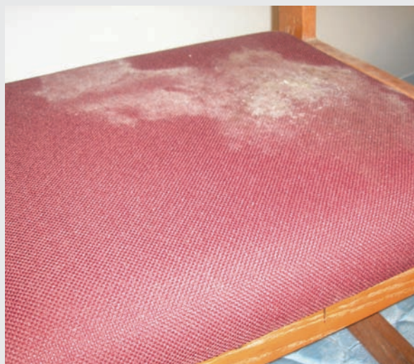
Figure 2.3-B Mold Growth due to Negative Pressure
